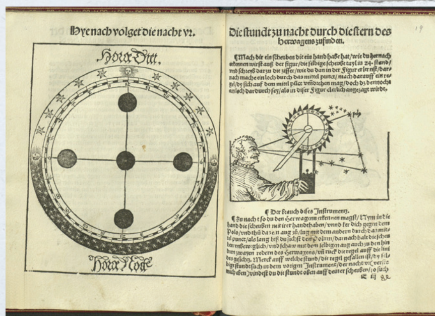
Cut-out disc to make a revolving diagram of the stars, complete with instructions for construction and use. Peter Apian, Ein Kunstlich Instrument (1524). Beinecke Rare Book and Manuscript Library (Taylor 59).
